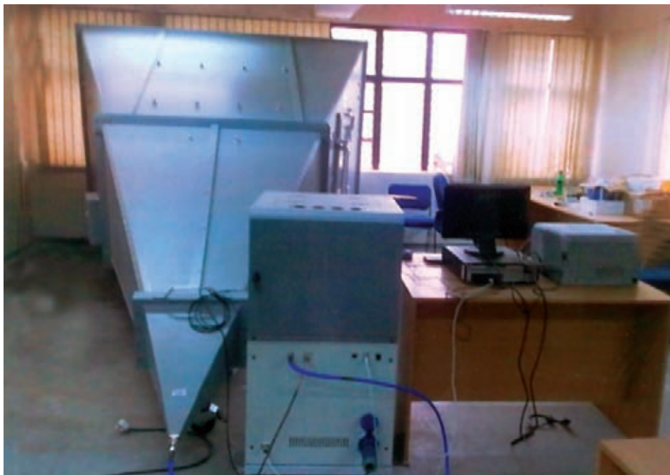
GTEM Machine installed at RRSLs for Electronic Test of Equipments
