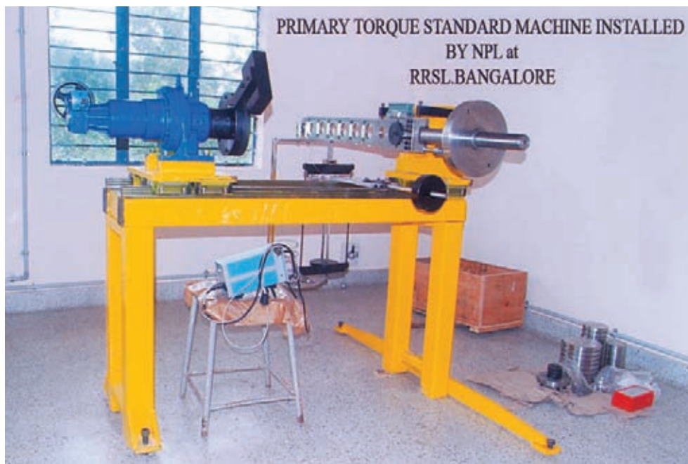
Primary Torque standard machine installed by NPL at RRSL, Bengaluru
