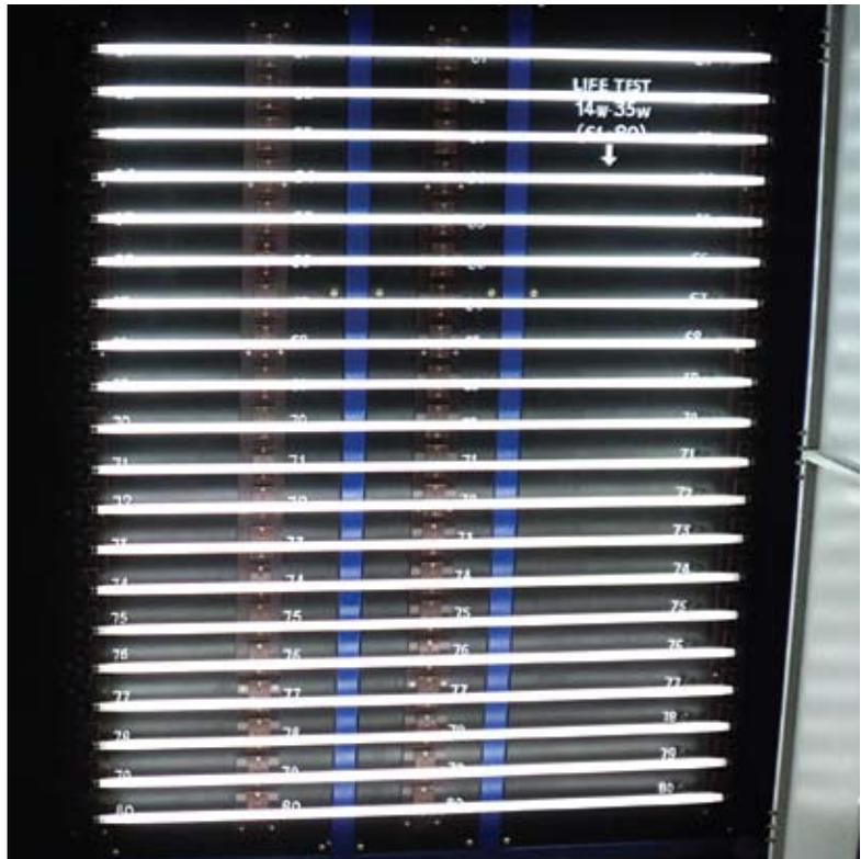
Life Test in progress at Testing Laboratory
